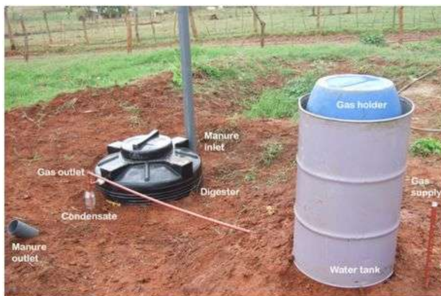
Figure 21 Demonstration biogas system established by the project in Mozambique.
