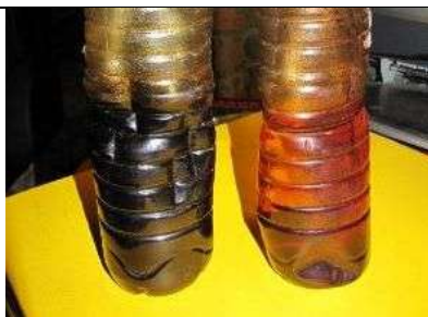
Fig 2 Cotton oil, before treatment left, acidity 20.4 after treatment right, acidity 0.08.
