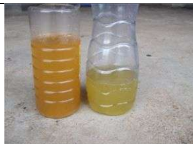
Fig 1 Jatropha oil, before treatment left, acidity 17, after treatment right, acidity 3
