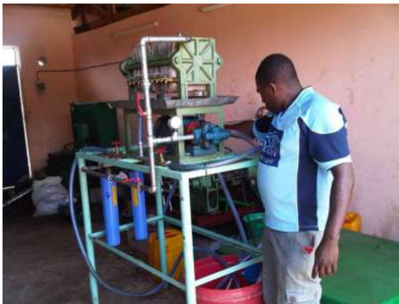
steel tanks with compartments (Mozambique) can be used for sedimentation as a first step. Figure 17 Filtering Jatropha oil, Bilibiza, Mozambique.
