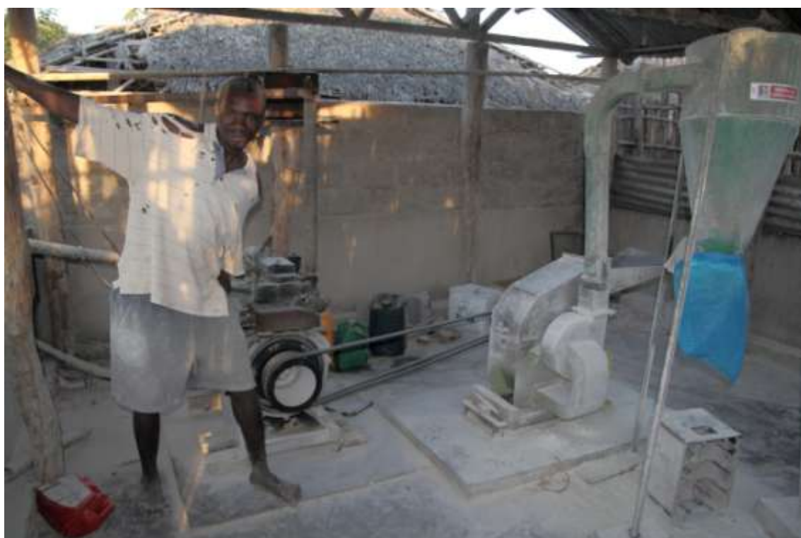
Figure 4 Local maize mills like this one can be converted to run on Jatropha oil.
