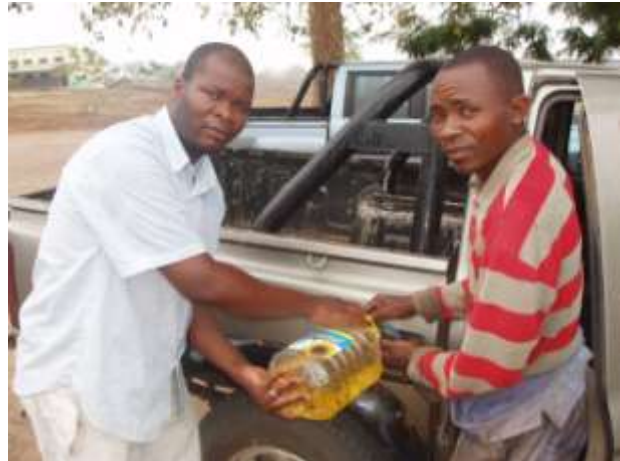
Figure 19 Fueling the modified Nissan in Mozambique with cooking oil.
