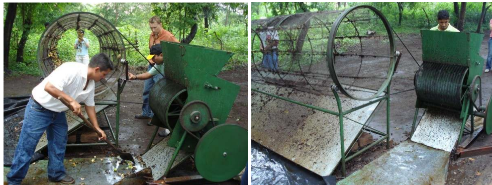
De-husker as observed in Nicaragua (Tempate project) and replicated in San Martín by the CFC-DED project. After crushing the fruits, separation of seeds and husks is done by a rotating shaft with wire netting through which the seeds fall down while the husks accumulate at the end (Photos: Martijn Veen, August 2008).
