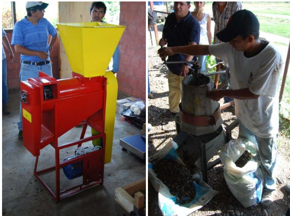
De-husking machines as being applied in San Martin. To the left, a model from Brazil as introduced in San Martin by Agrobiofuels Peru and replicated by a local technological institute, issues by DRASAM. To the right, the Universal Nut Sheller as developed by The Full Belly Project (US) for manual use at farm level by small-holders (photo from Honduras but soon will be introduced in San Martin).
