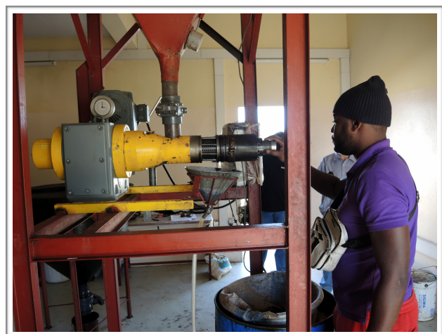
Figure 5.9: THD oil press, an AXIA 4 KW model with 50,000 l/yr capacity
